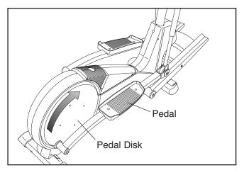
To dismount the elliptical crosstrainer, wait until the pedals come to a complete stop. Note: The elliptical crosstrainer does not have a free wheel; the pedals will continue to move until the flywheel stops. When the pedals are stationary, step off the highest pedal first. Then, step off the lowest pedal.
